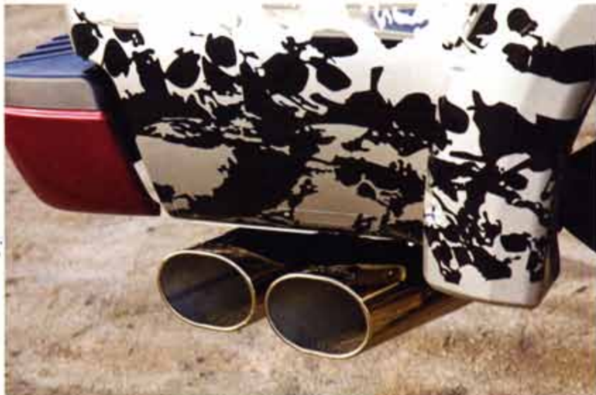
For enhanced diesel performance, products from Gale Banks were installed, including an air cleaner, intake and cat-back exhaust with stainless steel tips.
