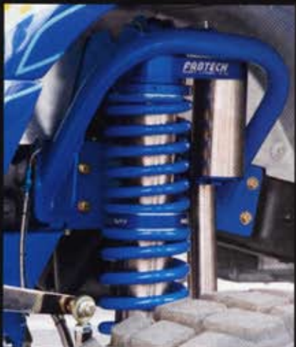
▲ Dirt Logic 4.0 Coilover shocks from Fabtech control the ride.
