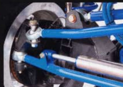
▲ Hydraulic ram-assist steering from Howe controls the front.
