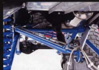
▲ A custom-designed three-link suspension is used on the rear end.
