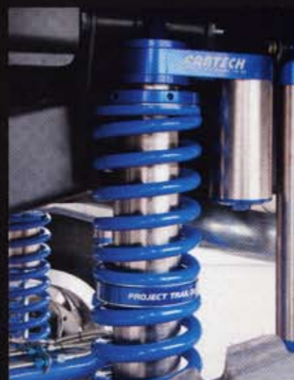
▲ Dirt Logic 4.0 coilover shocks control the ride at the rear of the truck.
