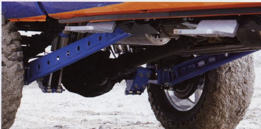
▼ The rear suspension is as beefy as the front, resulting in an 8-inch overall lift.
