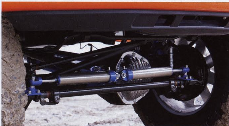
▲ The Fabtech Ford's four-link setup uses 2-inch tubing with 1-inch spherical ball endlinks for incredible strength.
