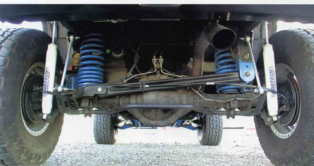
The Fabtech suspension system gives the H2 not only a 6-inch lift over stock, it also gives it the ability to tackle whatever bumps in the road Mother Earth throws at it.
