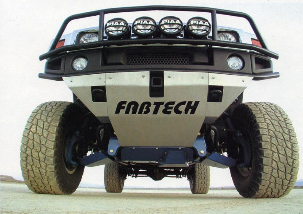
The front end of the H2 is all business, thanks to the huge Fabtech skid plate and custom-made front desert guard. Providing plenty of candlepower are the multiple PIAA auxiliary lights mounted into the guard.
