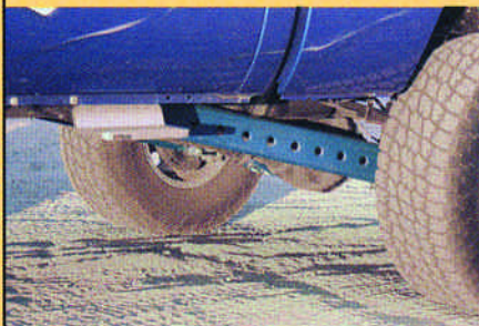
▲ Fabtech's powercoated dual shock hoops are gusseted for strength and backed by hand-fabricated aluminum inner fenders. The new fenders were constructed after the stock ones were trashed and the new fiberglass frontend was installed.
