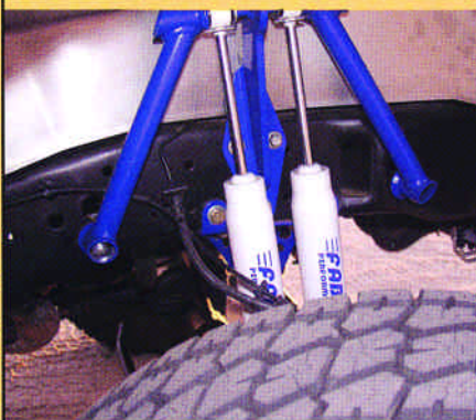
▲ Fabtech's powercoated dual shock hoops are gusseted for strength and backed by hand-fabricated aluminum inner fenders. The new fenders were constructed after the stock ones were trashed and the new fiberglass frontend was installed.
